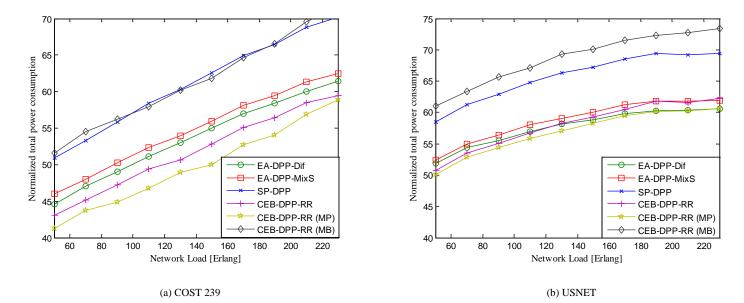
Fig. 4. Normalize power consumption of the network in various offered load, (a) COST 239, (b) USNET
