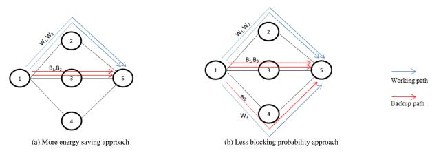
Fig.1. Example of survivable green routing to trade-off between energy saving and blocking probability
