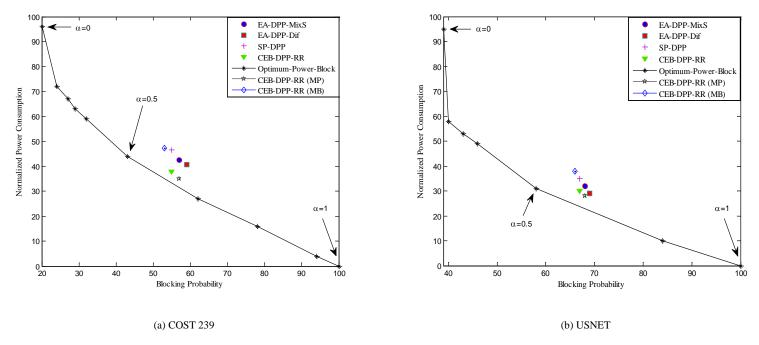
Fig. 7. Pareto-optimal frontier of power consumption and blocking probability and comparison with heuristic algorithms in 100 Erlangs, (a) COST 239, (b) USNET
