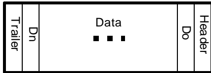
Fig. 3: Transfer flit structure
