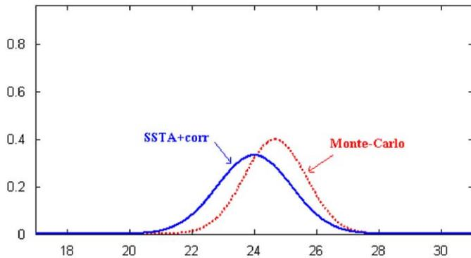
Fig. 6. Comparison of SSTA (with Correlation) and MC methods: PDF curves.
