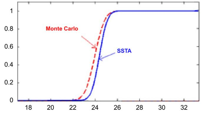
**Fig. 5.** Comparison of SSTA and MC methods: CDF curves.
