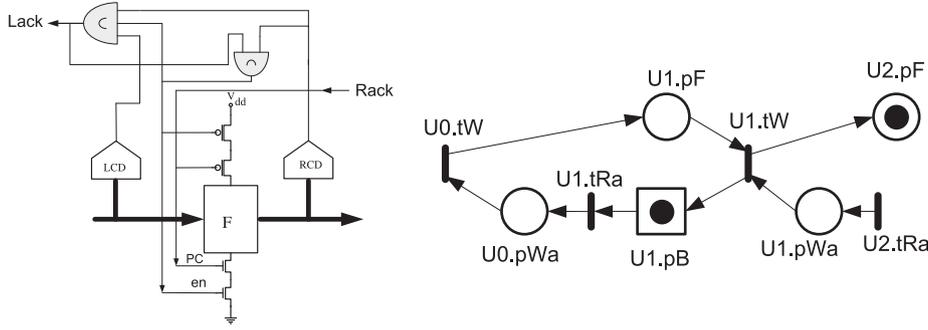
Fig. 2. A simple Full Buffer Template and its Corresponding Timed Petri-Nets model.
