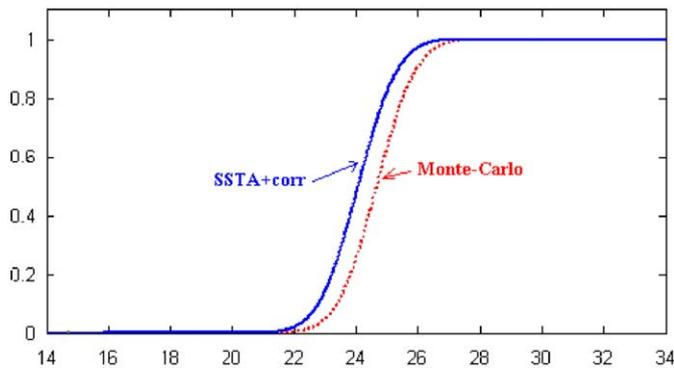
Fig. 7. Comparison of SSTA (with Correlation) and MC methods: CDF curves.
